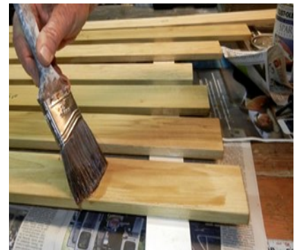
Wood slats are double coated with varnish on all sides.
